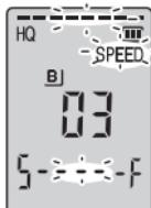
The playback speed rises as the flashing bars move right. The illustration shows the display for the normal speed playback.
